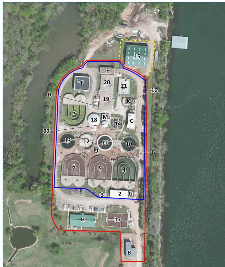
Figure 1 – Permanent flood wall alignment (red line).
