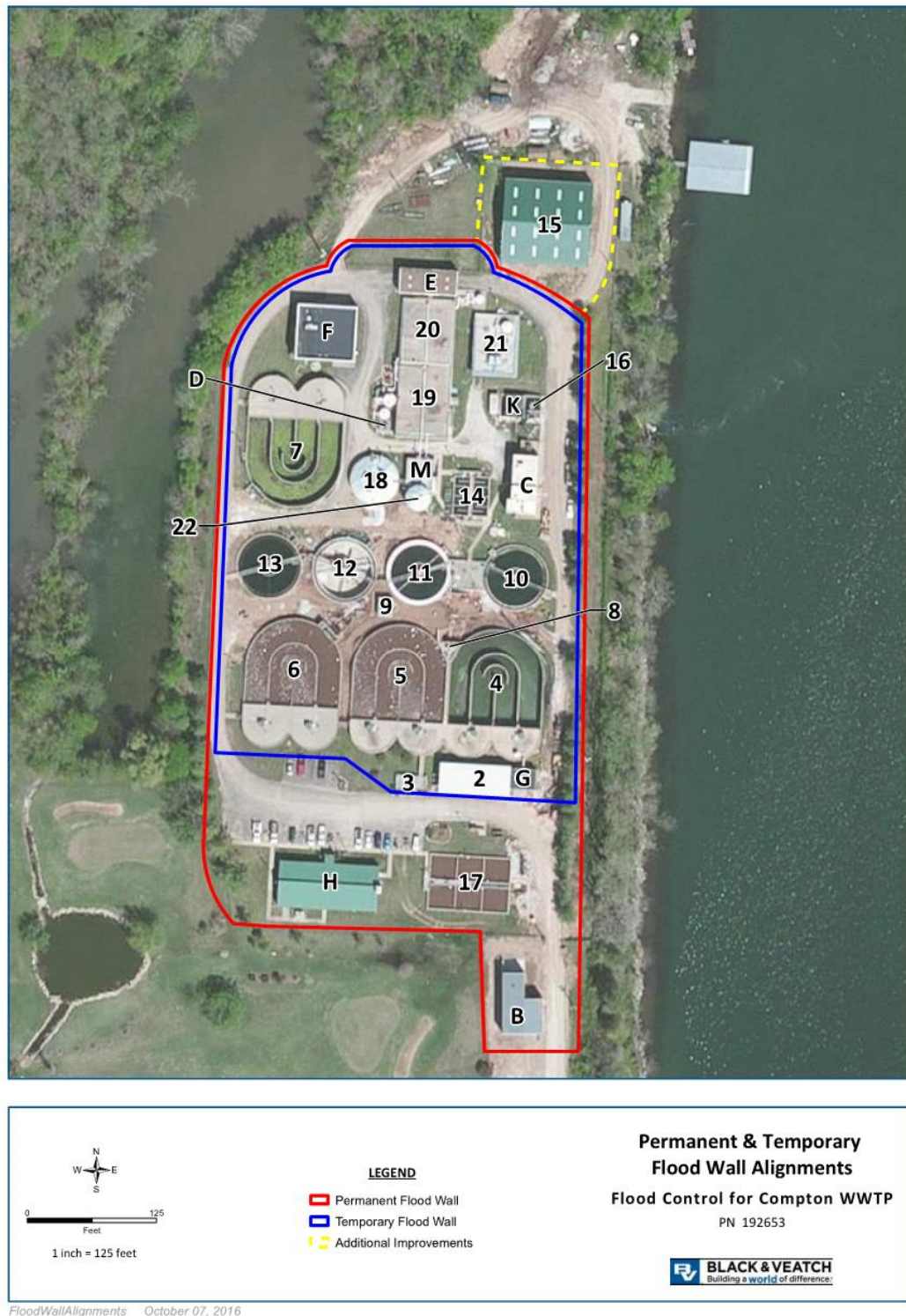
Figure 1-3 Permanent and Temporary Flow Wall Alignment Layout
